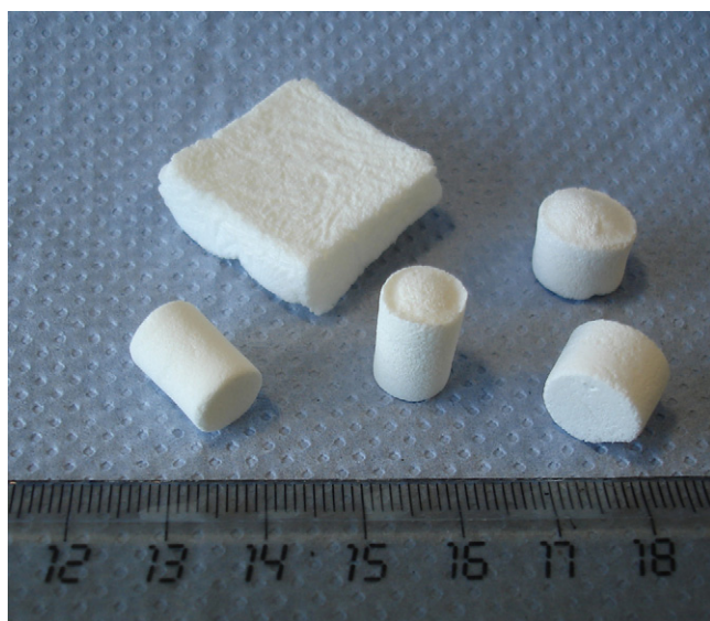
Fig. 1. Porous scaffolds, made from mineralised collagen, in different size and shape (the scale shows centimetres).
